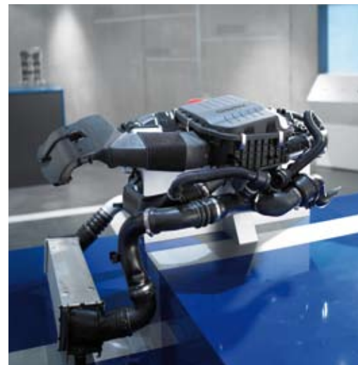
Complete air intake system, including intake air passage, filter, intake module, parallel arrangement of an exhaust gas turbocharger, charge air lines including charge air cooler, sound generator, and cylinder head cover with integrated oil mist separation.
