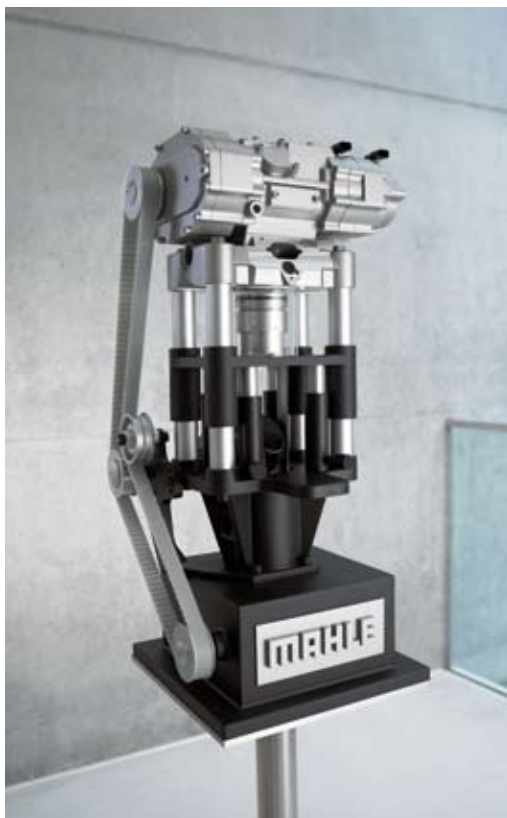
1-cylinder research engine with optical access to the combustion chamber in the cylinder head and cylinder, with high-strength quartz cylinder liners and pistons with sapphire glass bottom.
