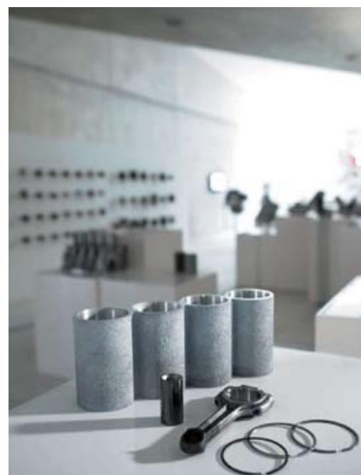
ALBOND® cylinder liner compound with minimal land widths between cylinders; piston pin with DLC coating; weight-optimized forged cracked conrod with small, stepped pin end bore and manganese-phosphate coating; piston rings.
