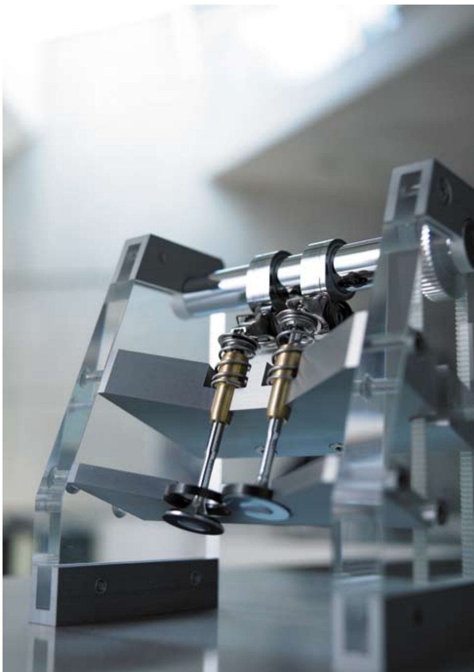
Cylinder deactivation // Cylinder deactivation to increase efficiency and decrease friction losses.
