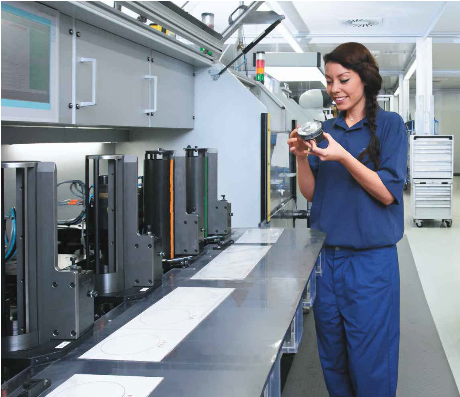
Employee setting up an automated piston measurement and piston ring assembly device
