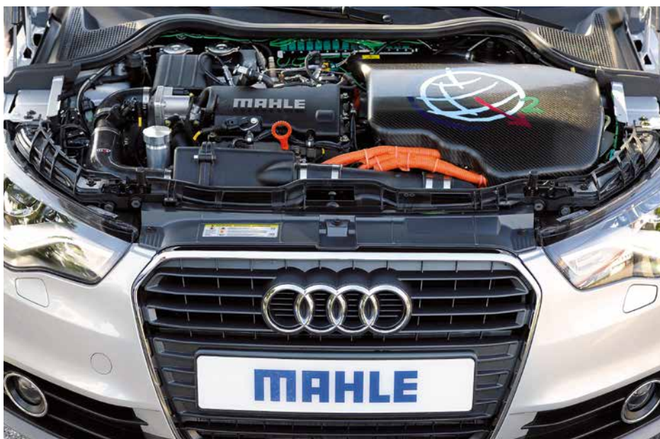
Top: the MAHLE range extender drive achieves efficiency of up to 31 percent.
