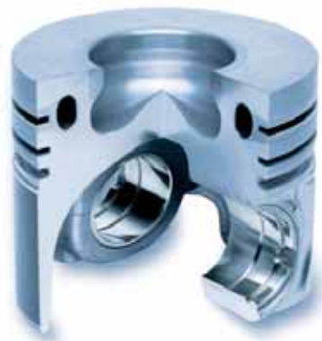
Piston for passenger car diesel engine with cooled ring carrier and fiber-reinforced combustion bowl rim
