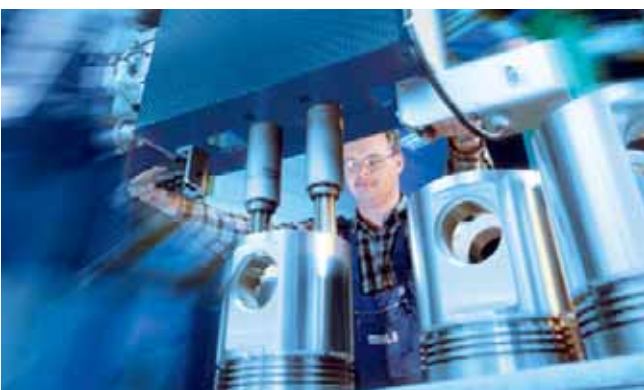
Electronically controlled tightening of piston screws in the final assembly
